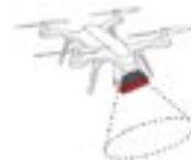
Both sensors have to be firmly held to limit vibrations during the flight. Their holding has to be consolidated. **Their movement must be in unison**, the change in one's orientation must be reflected in the other **such that the angle between their planes remains constant.**
