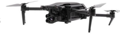
2025 : ANAFI UKR & CHUCK 3.0 fully autonomous IA based ISR micro-UAV
