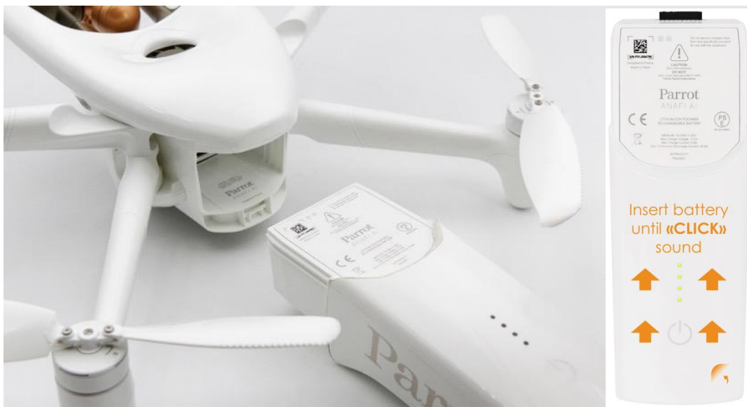
ANAFI Ai: battery ready for installation
