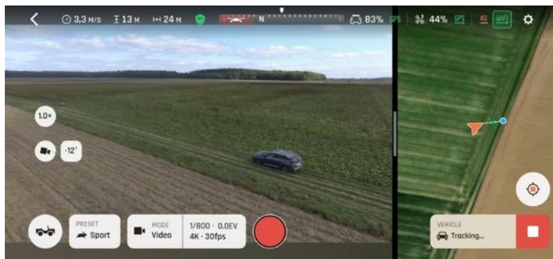
Tracking in progress, no command from the pilot: ANAFI Ai is travelling as the same speed as the vehicle
