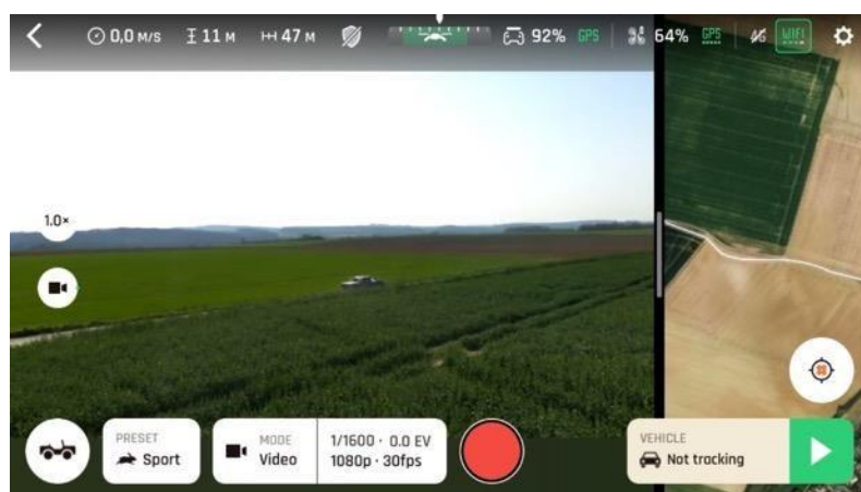
Tracking suspended, no command from the pilot: ANAFI Ai is hovering
